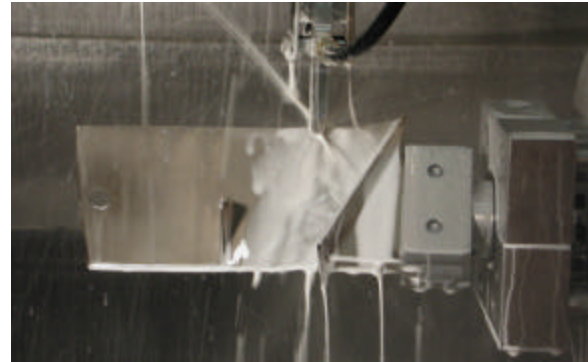
Figure 6 – First stage fan blade being LPB processed in 4-axis CNC facility.
