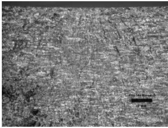
Figure 7: Fracture face showing typical surface failure for milled specimen.
