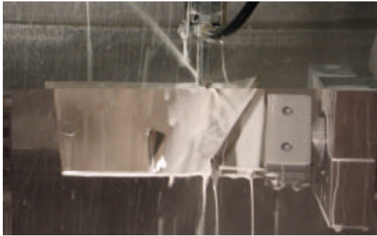
Figure 6 – First stage Ti-6-4 fan blade being LPB processed in 4-axis CNC facility.
