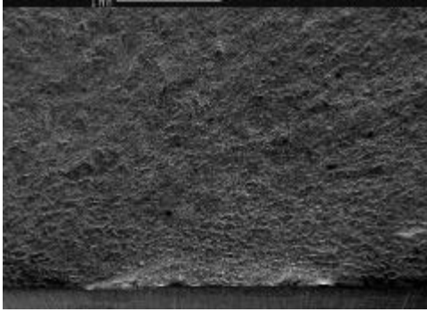
Figure 4a: Fracture surface showing multiple initiation sites.
